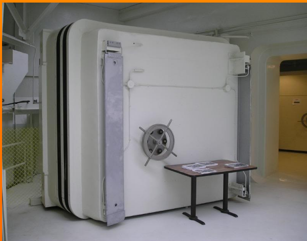
High Pressure/Vacuum Space Test Facility - Dual Pneumatic Seals and Hydraulic Operation
